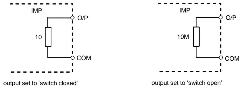
**Fig 9.8** Equivalent circuits of the digital outputs.
